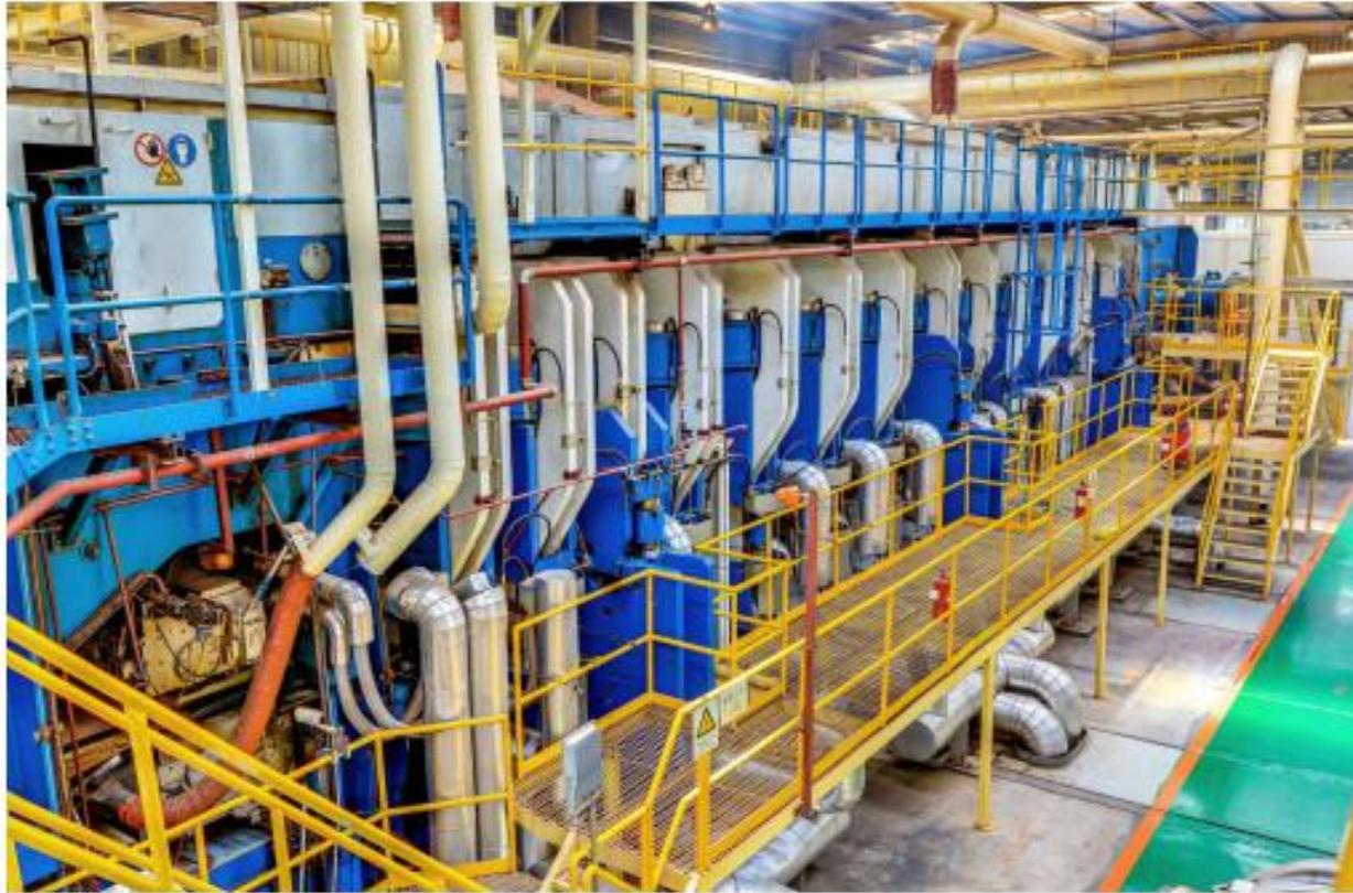
compress the suitable mat under simultaneous influence of pressure ,temperature , speed and other parameters ,manufacturing thickness-setted particleboard
